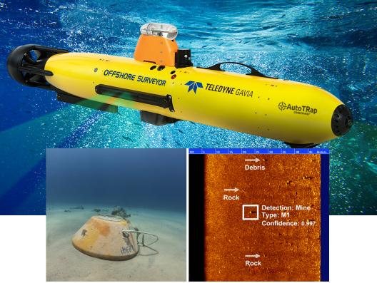
AutoTRap Onboard® empowers your autonomous underwater vehicle (AUV) to act on real-time sonar data to detect objects on the seafloor. The app then provides contact alerts to your system and allows your AUV to investigate further on its own—there's no need to surface, review data, and re-deploy it with a new mission.
