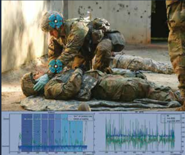
MEDIC uses fNIRS sensors mounted to a medic's helmet to measure indicators of cognitive load. A body-band device includes additional sensors to measure indicators of physical activity.
